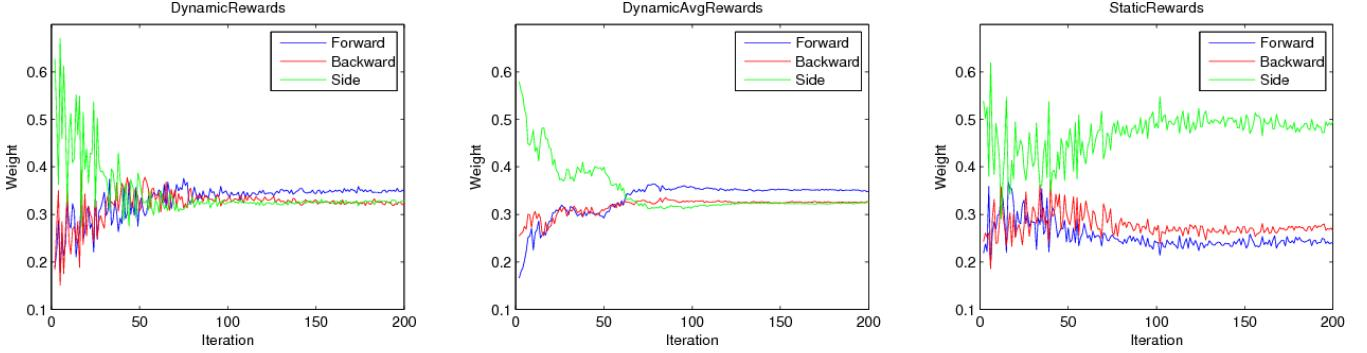
**Figure 5:** Directional reward weights during the course of optimization for the the *DynamicRewards* agent (left), *DynamicAvgRewards* agent (center), and *StaticRewards* agent (right). Note that the weights used by the *StaticRewards* agents are fixed and that the weights shown in this figure are only computed and displayed for comparison purposes to show what the weights chosen would be if the agent was dynamically adjusting its weights. Higher weights correlate to lower relative rewards.
