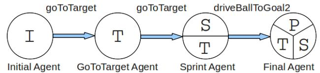
**Figure 3: UT Austin Villa walk parameter optimization progression.** Circles represent the set(s) of parameters used by each agent during the optimization progression while the arrows and associated labels above them indicate the optimization tasks used in learning. Parameter sets are the following: I = *initial*, T = *goToTarget*, S = *sprint*, P = *positioning*.
