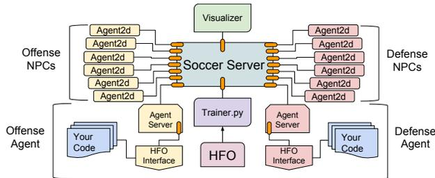
**Figure 2: The HFO Environment is comprised of many separate processes which communicate over the network with the RoboCup 2D soccer server. HFO starts these processes, ensures they communicate, and oversees the games. A user needs only to specify the number of offensive and defensive agents and NPCs and then connect their agent(s) to the waiting Agent Server(s) via the HFO interface.**
