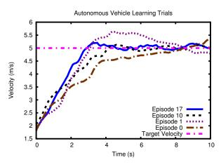
Fig. 10: Control profiles of learning trials performed on the physical vehicle.
