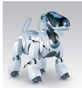
Fig. 1. A Sony Aibo ERS-7. The arrows point to the shoulder (1), abductor (2), and knee joint (3) of the Aibo’s right front leg.
