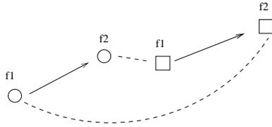
**Fig. 3.** A case in which greedy association fails but global optimal association performs well. The arrow indicates the actual object displacement over subsequent frames f1 and f2. The dotted lines indicate the wrong matches returned by greedy association.
