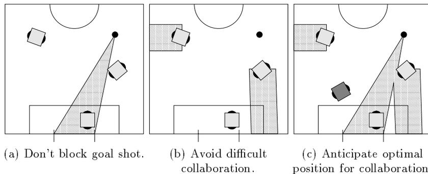
**Fig. 9.** Constraints for the dynamic anticipation algorithm are represented as shaded regions; (a) and (b) show three opponents and the current position of the ball; (c) illustrates the position of the passive agent - dark square - as returned by SPAR.
