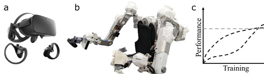
**Figure 1.** We observe the effect of learning in (a) the task space (score and end effector speed) measured in a virtual task environment, and (b) the joint space (joint angles, velocities, and torques) measured using the Harmony exoskeleton's sensors. The expected trends in performance change over the course of training seen in (c) may vary, but participants are all expected to improve and become experts crossing a threshold performance level.
