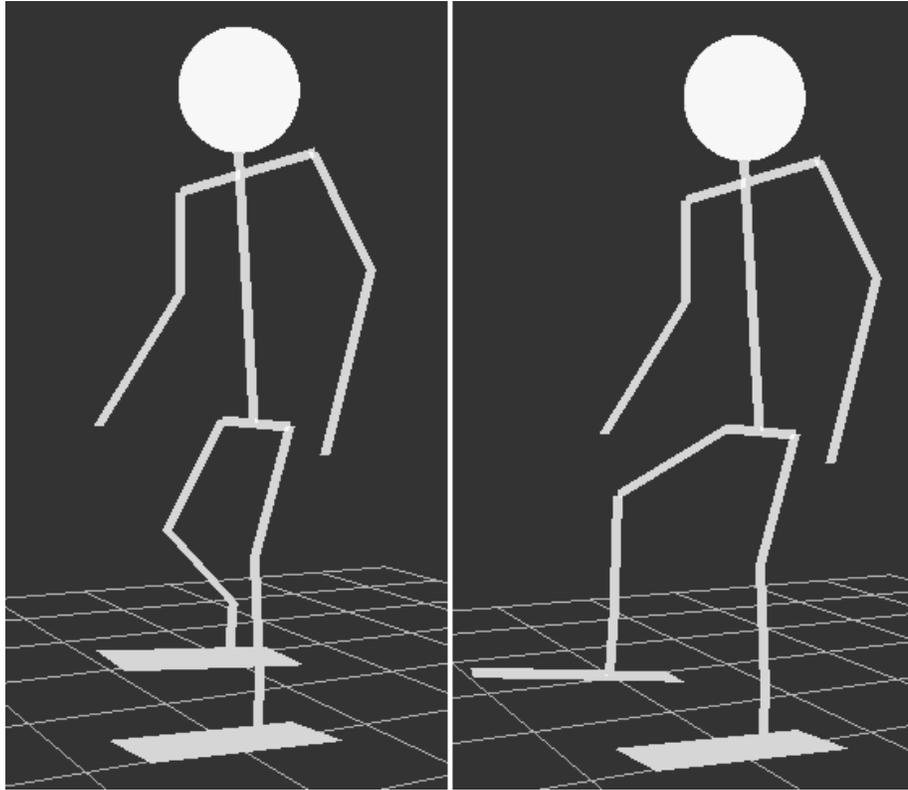
Figure 9: This figure shows a model of a robot in Webots kicking the ball. State 2, where the robot brings its leg back, is shown on the left. State 3, where the robot swings its leg forward, is on the right.
