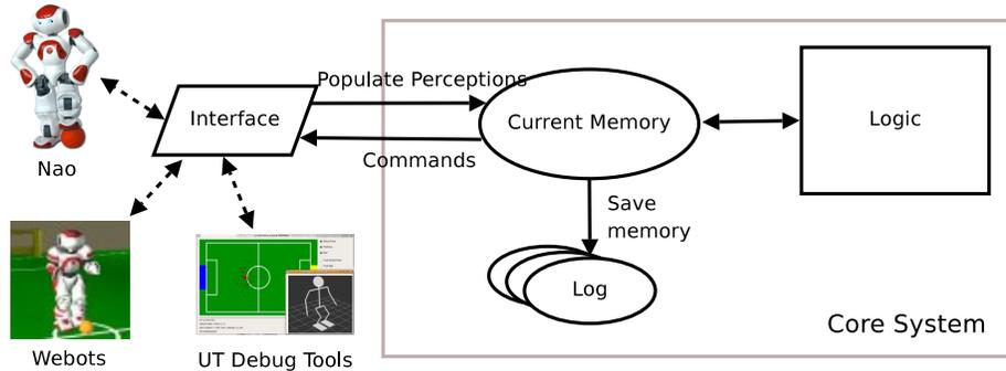
Figure 2: Overview of the 2008 UT Austin Villa software architecture.
