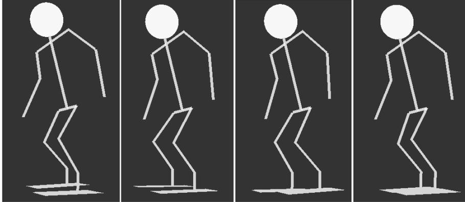
Figure 8: This figures shows the states in our walk engine. In the first state, the robot shifts its weight to its left leg and lifts its right leg. In the second state, it rebalances its weight and brings the right leg forward and down. In states 3 and 4, the robot repeats this motion with the legs reversed.
