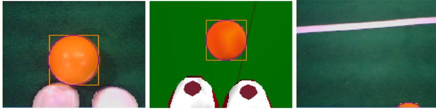
Figure 5: Example of circle fitting applied to the ball. The first two images are examples of a ball when the robot is preparing to kick (an image is presented from the robot and from the simulator). The third image shows a ball where circle fitting is required to get an accurate estimate of distance.
