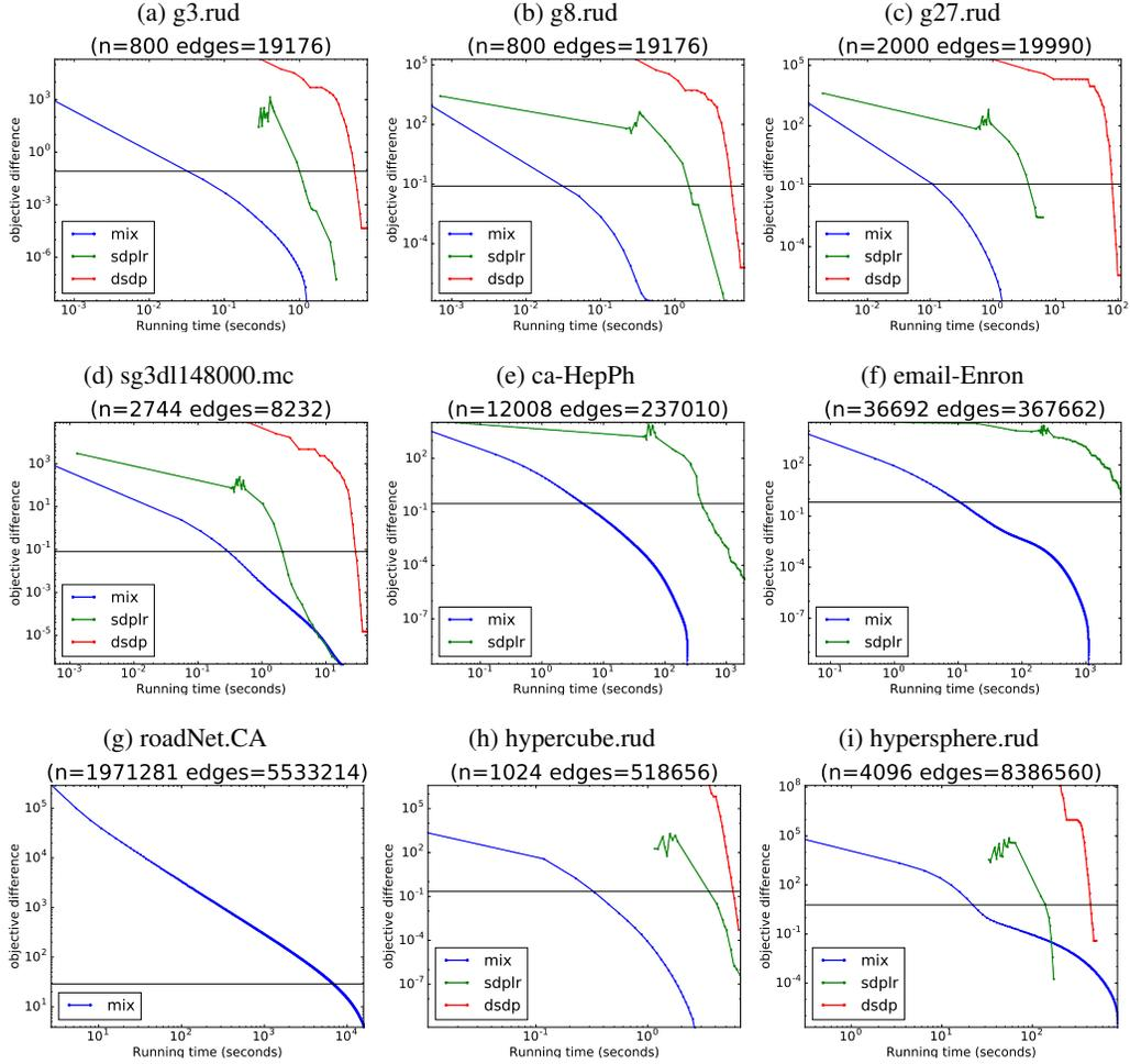
Figure 1: The log-log plots of function difference  $f(x) - f^*$  v.s. running time in seconds. The horizontal line marks  $1e - 4$  times the initial function difference of the MIXING method.
