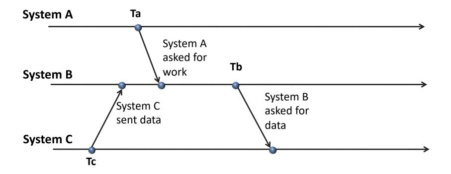
• But in reality, we do not know if Tc occurred **before** Ta and Tb, because in an asynchronous distributed system **clocks are not synchronized**!
