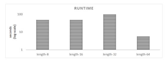
Figure 3: Runtime of Verilog implementation running in Cascade software mode on inputs of length 8,16,32,64. NOTE: the data in this graph are random. If your data are different that's GOOD.
