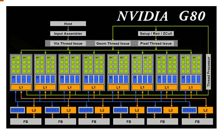
Mapping to Graphics pipeline no longer apparent Processing elements no longer specialized to a particular role Model supports *real* control flow, larger instr count
