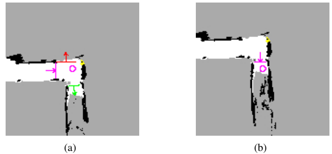
Fig. 11. Low light causes floors to appear texture-less leading to poor stereo distance information. (a) The robot arrives at the T intersection in Figure 12(a). The right (downwards facing) hallway is poorly lit. (b) As the wheelchair travels down this hallway it quickly arrives at the “frontier” of free space since the dark floor remains unseen (and incorrect distance information leads to phantom obstacles). This results in no gateways facing down the hall causing the wheelchair to believe it is at a dead end.
