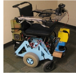
Fig. 1. The current Intelligent Wheelchair platform. A human “driver” can either use the joystick or GUI interfaces via a laptop. There is a stereo camera on a pan-tilt unit, one horizontal lidar, and one vertical lidar (currently unused). The horizontal lidar is used for efficient SLAM; however, future platform configurations should eliminate expensive lidar sensors and utilize visual SLAM [3] along with the visual 3D modeling discussed below.
