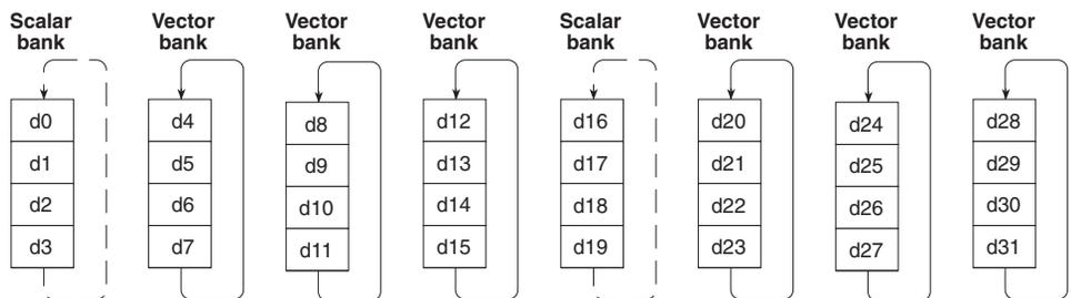
Figure F-2 Register banks, 32 double-precision register VFP
