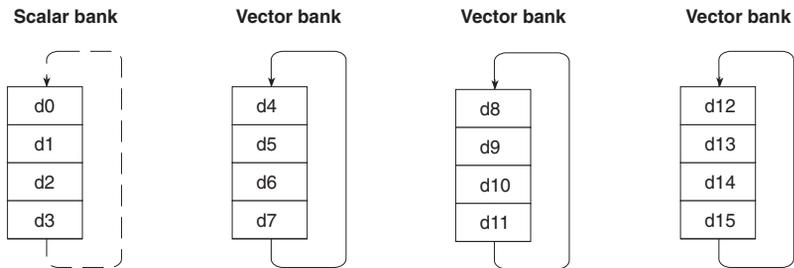
**Figure F-3 Register banks, 16 double-precision register VFP**
