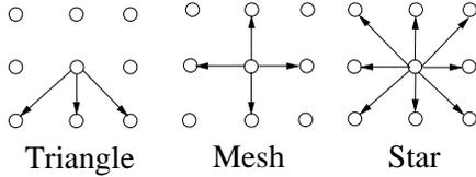
Figure 5: Multi-hop GPA Interconnects. Only the wires out of the center node of the representative 3x3 array is shown.
