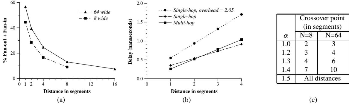
Figure 2: Percentage wire delay contribution, total communication delay. The table shows the crossover point for single-hop and multi-hop networks. The crossover point indicates the maximum distance communication for which multi-hop networks are better.
