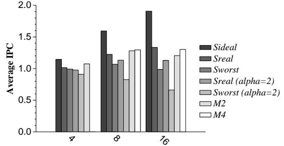
Figure 4: VLIW IPC averaged across the high IPC benchmarks *dct*, *mpeg2encode* and *radar*.
