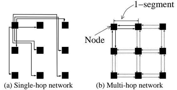
Figure 1: Single-hop and multi-hop networks of size 9. Only wires corresponding to the top left node are shown for (a).
