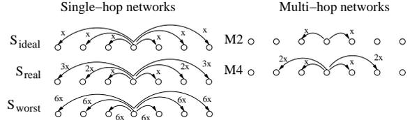
Figure 3: VLIW interconnect networks. The scaling factors on the arcs refer to the relative delays of the wires based on the distance traveled.
