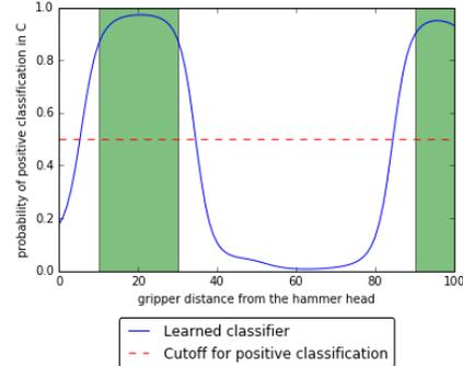
Fig. 7. Classifier: robot can grip the hammer between the 10<sup>th</sup> and 30<sup>th</sup> or 90<sup>th</sup> and 100<sup>th</sup> gripper locations
