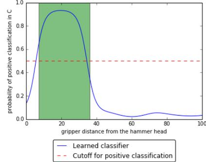
Fig. 6. Classifier: robot can grip the hammer between the 7<sup>th</sup> and 36<sup>th</sup> gripper locations
