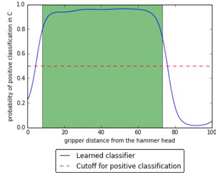
Fig. 5. Classifier: robot can grip the hammer between the 8<sup>th</sup> and 73<sup>th</sup> gripper locations
