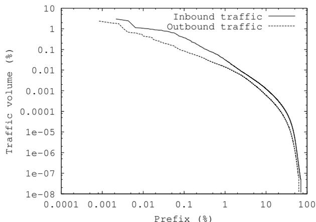
Fig. 4. Fraction of traffic vs. fraction of prefixes
