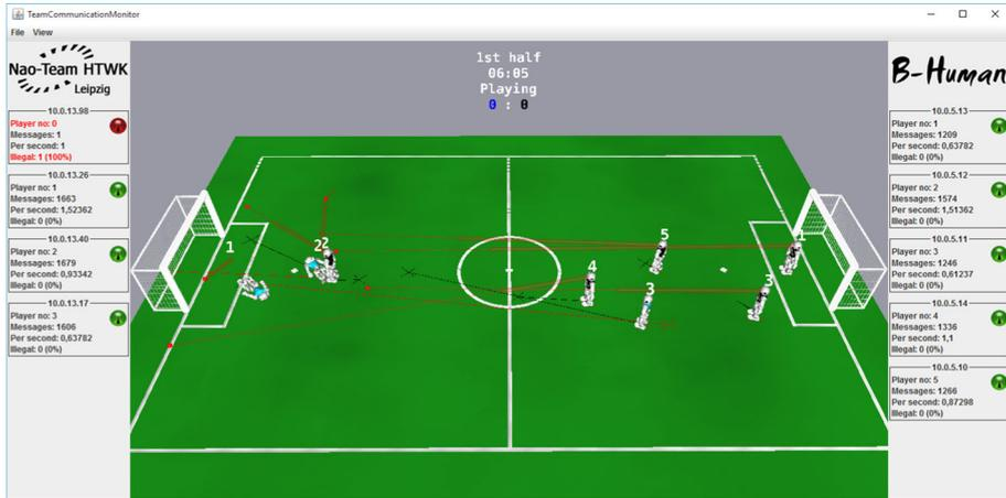
**Fig. 2** Team Communication Monitor during a normal Standard Platform League game. The centered 3-D view displays the current world states, i.e. position, status, and ball position, communicated by the playing robots. The side views show the status and the frequency of each robot's communication
