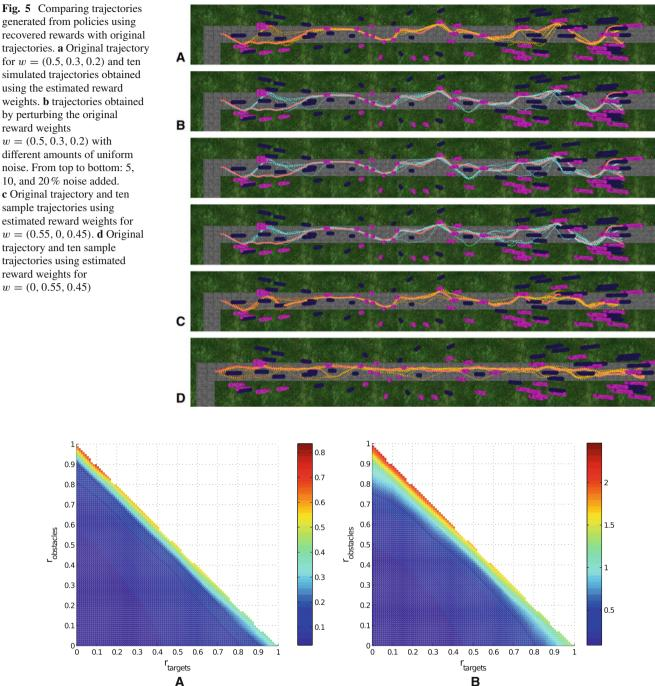
Fig. 6 Error in the trajectories. a Mean squared deviation between trajectories obtained with the same reward weights. b Mean squared deviation between the demonstrator's trajectory and trajectories obtained from the estimated weights
