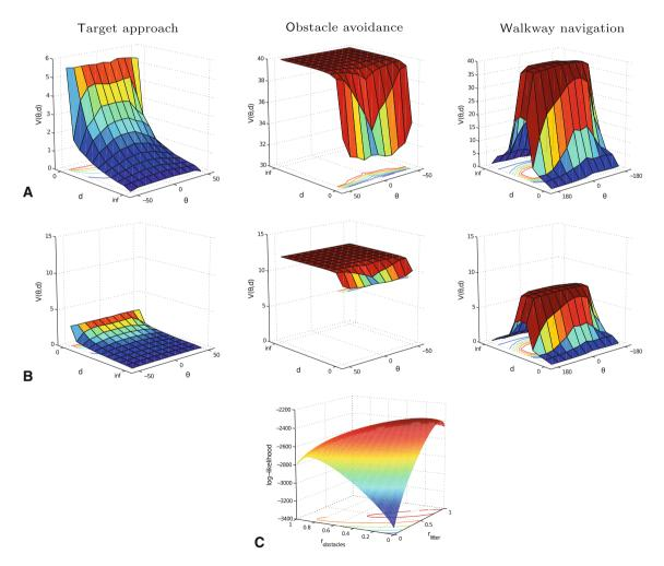
Fig. 3 a The value functions obtained for a reward of one unit. b The scaled value functions as recovered by the IRL algorithm, where the weights for the tasks are represented as (target approach, obstacle avoid-
