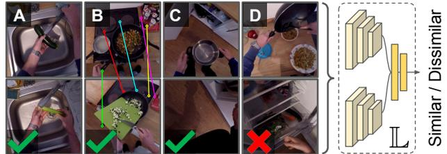
**Figure 2: Localization network.** Our similarity criterion goes beyond simple visual similarity (A), allowing our network to recognize the stove-top area (despite dissimilar features of prominent objects) with a consistent homography (B), or the seemingly unrelated views at the cupboard that are temporally adjacent (C), while distinguishing between dissimilar views sampled far in time (D).
