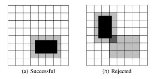
Figure 2: (a) The vehicle's space-time request has no conflicts at time t. (b) The black vehicle's request is rejected because at time t of its simulated trajectory, the vehicle requires a tile already reserved by another vehicle. The shaded area represents the *static buffer* of the vehicle.
