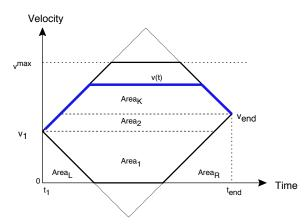
(a) Case 1: Area<sub>L</sub> + Area<sub>R</sub> + Area<sub>1</sub> + Area<sub>2</sub>  $< D \leq$  Area<sub>L</sub> + Area<sub>R</sub> + Area<sub>1</sub> + Area<sub>2</sub> + Area<sub>3</sub>
