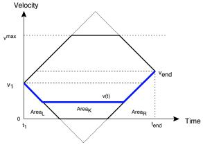
(c) Case 3: Area<sub>L</sub> + Area<sub>R</sub>  $\leq D \leq$  Area<sub>L</sub> + Area<sub>R</sub> + Area<sub>1</sub>
