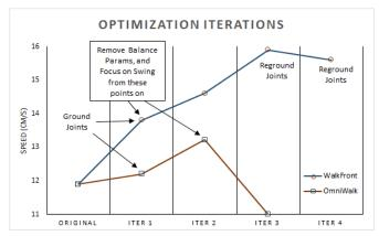
Figure 4: The performance of parameters through iterations of the GSL algorithm, and the guidance used to achieve these results.
