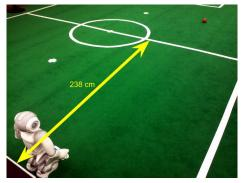
Figure 3: To evaluate the robot, it was placed in the position shown in this image and was ordered to walk towards the orange ball. Once it reached the center line of the field, it was ordered to stop, at which point it recorded its own walking time.
