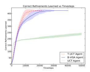
Figure 4: A comparison of T-UCT, B-VISA, and UCT agents on the light box domain [10]. The data show the number of timesteps required for the agents to learn all of the 424 CPT refinements needed to model the domain, averaged over 25 trials. Shaded regions represent standard error.
