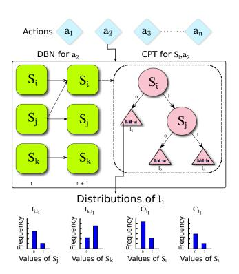
Figure 1: Top: All actions available in the environment. Left: A DBN representing the effects of action  $a_2$  on state variables  $S_i, S_j, S_k$ . Right: The CPT encoding transition dynamics for state variable  $S_i$ under action  $a_2$ , with leaves labeled with distributions. Bottom: The distributions of values that are tracked at leaf  $l_1$  (see Section 2.3).
