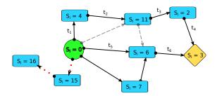
Figure 2: A full transition graph  $\mathcal{T}_i$  (all edges) and its randomized subgraph  $T_i$  (solid edges), as described in Section 3.3.  $T_i$  represents a set of possible paths for  $S_i$  from a source value  $S_i = 0$  to a target value  $S_i = 3$ . The dotted lines represent a dead end. The dashed lines represent transitions in  $\mathcal{T}_i \setminus T_i$ .
