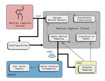
Figure 1: Control flow of the MARIONET Interface
