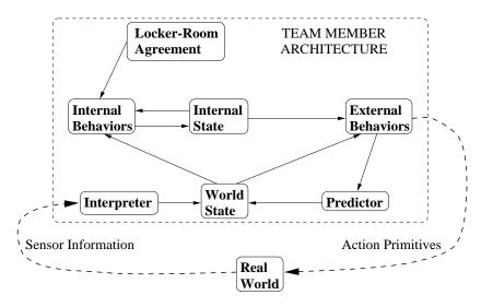
Figure 1: A functional input/output model of the team member agent architecture for PTS domains.
