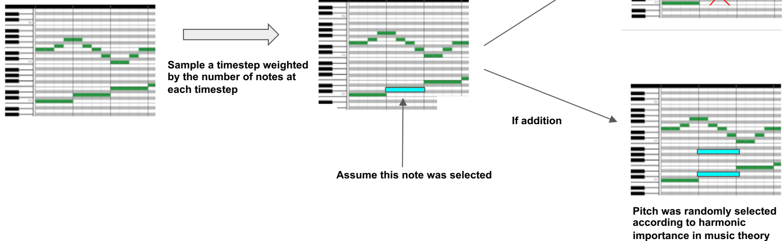
Fig 7. We designed a method that can automatically generate harmonic intervals and automatically remove notes. To add notes, the algorithm requires two steps. First we sample harmonic intervals from a probability distribution computed from aggregating music theory rules used in prior work.
