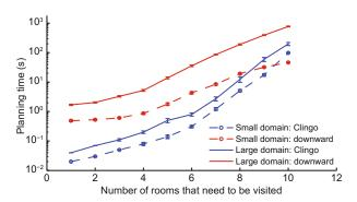
Fig. 1 Robot navigation: small domain, 10 rooms; large domain, 15 rooms. Forty percent of rooms are connected via doors, and the rest are directly accessible from the corridor
