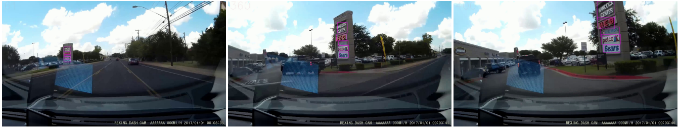
Figure 2: In a challenging driving scene, the vehicle’s motion changes the location and dimensions of the points of interest relative to the human within the vehicle. The points of interest in this figure are marked by magenta bounding boxes.
