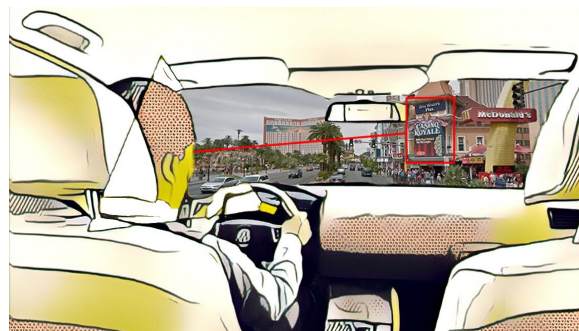
Figure 1: A use case of intention inference. In the setting of a human driver riding in a vehicle, a DMC captures the driver gaze, and a road camera captures the street view. Based on the captured images, an autonomous agent infers which point of interest in the street view that the driver is interested in going toward or obtaining more information about.
