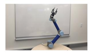
Figure 2. The UR5 Robot Arm
