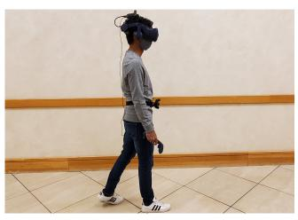
(b) Participants wear an HTC Vive Pro Eye head-mounted display with a WiGig wireless adapter and an HTC Vive Tracker on a belt mounted to the waist. They interact with controls in the experiment using the Vive Controller.
