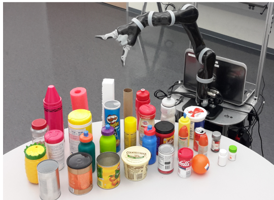
Figure 1: The robot used in our experiments, shown here with the 32 objects it explored in order to learn three ordinal properties: weight , width , and height .
