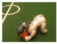
Fig. 1: An Aibo with control of a ball. Achieving this position without knocking the ball away in the process is a challenge; our learning method allows the Aibo to do this more reliably without sacrificing walking speed.
