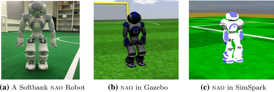
Fig. 3 The three robotic environments used here. The Softbank NAO is our target physical robot. The NAO is simulated in the Gazebo and SimSpark simulators. Gazebo is a higher fidelity simulator which we also use as a surrogate for the real world in an empirical comparison of grounded action transformation (GAT) to baseline methods
