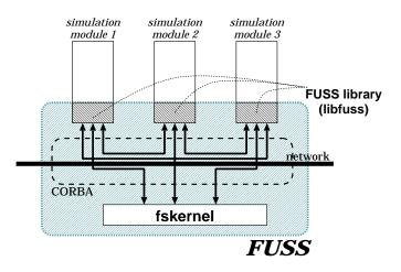
Figure 5. A Simulation System Built on FUSS
