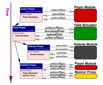
Figure 6. Phase Control and Communication with Joined Modules
