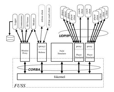
Figure 7. Design of the new soccer simulator
