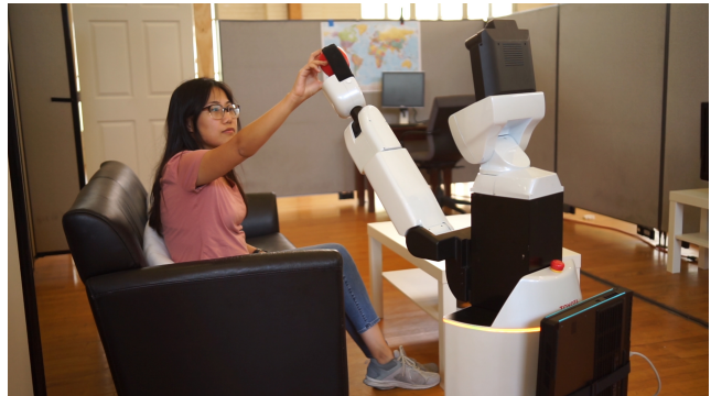
Figure 1: A Toyota Human Support Robot, representative of typical GPSRs, handing an apple to a user in a mock home environment.
