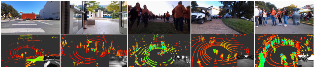
Fig. 2: Five example scenarios from SCAND showing the RGB image and below it the accompanying Lidar with the monocular image from side camera on the Spot. From left to right, the scenarios have the tags “Street Crossing”, “Narrow Doorway”, “Navigating Through Large Crowds”, “Vehicle Interaction”, and “Crossing Stationary Queue.”
