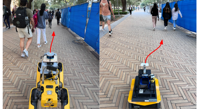
Fig. 1: A human demonstrator teleoperates the two robots, following a socially compliant strategy (left- moving with traffic, right- sticking to the right of the road) around human crowds.
