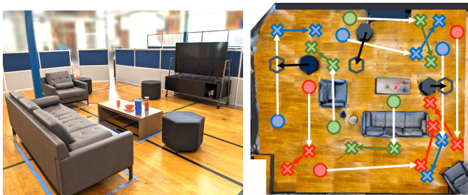
Fig. 5: Evaluation environment for Causal MoMa in the real-world. Left: The robot is placed in a mock apartment never seen during training and the best Causal MoMa trained policy is transferred zero-shot . Right: the robot is tasked with reaching different locations with the end-effector ( crosses ) from varying starting points ( circles ) while keeping a desired orientation, avoiding collisions, and keeping the goal in sight. We evaluate paths with three types of obstacles, no obstacles (red), static obstacles (green), and dynamic obstacles (blue) in the direct path to the goal, frequent in household environments. Each setup repeats for two types of goals, static and dynamic. First cross : robot’s initial end-effector goal (and final for static goals); Second cross : robot’s final end-effector goal, when the goal is dynamic. The policy trained with Causal MoMa achieves higher performance than a planning-based solution (with and without replanning) with privileged information about the layout of the scene.
