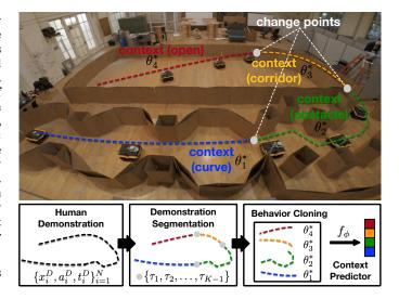
Fig. 1. Overview of APPLD: human demonstration is segmented into different contexts, for each of which, a set of parameters  $\theta_k^*$  is learned via Behavior Cloning. During deployment, proper parameters are selected by an online context predictor.
