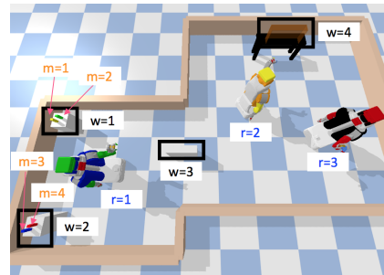
Fig. 1: Example MR-TAMP task showing the initial state. Robots ( \{r\}_{r=1}^3 ), movable objects ( \{m\}_{m=1}^4 ), and workspace regions ( \{w\}_{w=1}^4 ) are depicted in the figure, while fixed objects, corresponding to walls, shelves, table, and cabinet, are not shown. The goal is to move all movable objects from their initial locations to the cabinet ( i.e. , workspace region 4). The given task involves three robots such that robot 1 moves all movable objects to workspace region 3, and robots 2 and 3 move them to workspace region 4.
