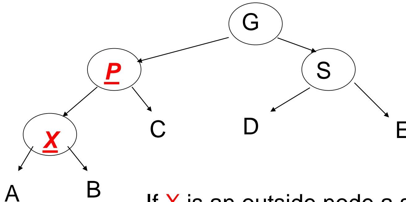
If **X** is an outside node a single *rotation* between **P** and **G** fixes the problem. A rotation is an exchange of roles between a parent and child node. So **P** becomes **G**'s parent. Also must recolor **P** and **G**.
