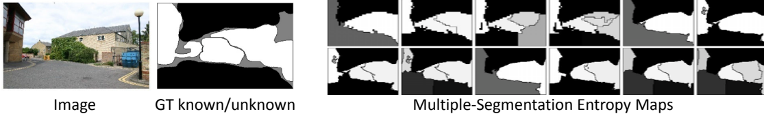
Figure 3. An example image, its ground-truth known/unknown label image, and our method’s predicted entropy maps for each of its 12 segmentations. For the ground-truth, black regions denote known classes (sky, road), and white regions denote unknown classes (building, tree). (Gray pixels are “void” regions that were not labeled in the MSRC ground-truth). In the entropy maps, lighter/darker colors indicate higher/lower entropy, which signals higher/lower uncertainty according to the known category models. Note that the regions with highest uncertainty (whitest) correspond correctly to unknown objects, while those with the lowest uncertainty (darkest) are known. Regions that are comprised of both known and unknown objects are typically scored in between (gray). By considering confidence rates among multiple segmentations, we can identify the regions that are least strongly “claimed” by any known model.
