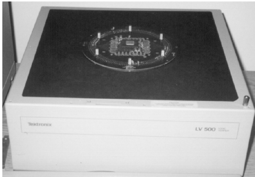
Figure 6: The LV500 Test Jig with the FM9001
