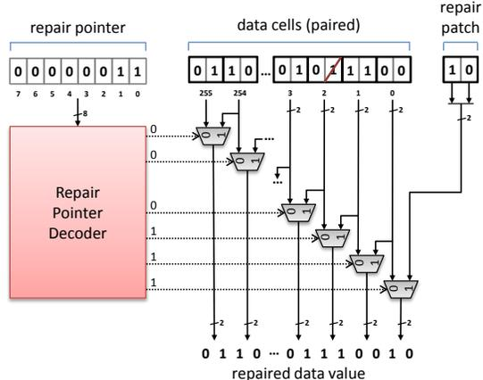
Figure 2: The “bit-fix” scheme proposed by Wilkerson *et al.*
