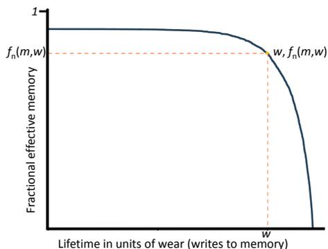
Figure 8: The fractional effective memory function plotted for ECP<sub>5</sub> with coefficient of variance 0.3.
