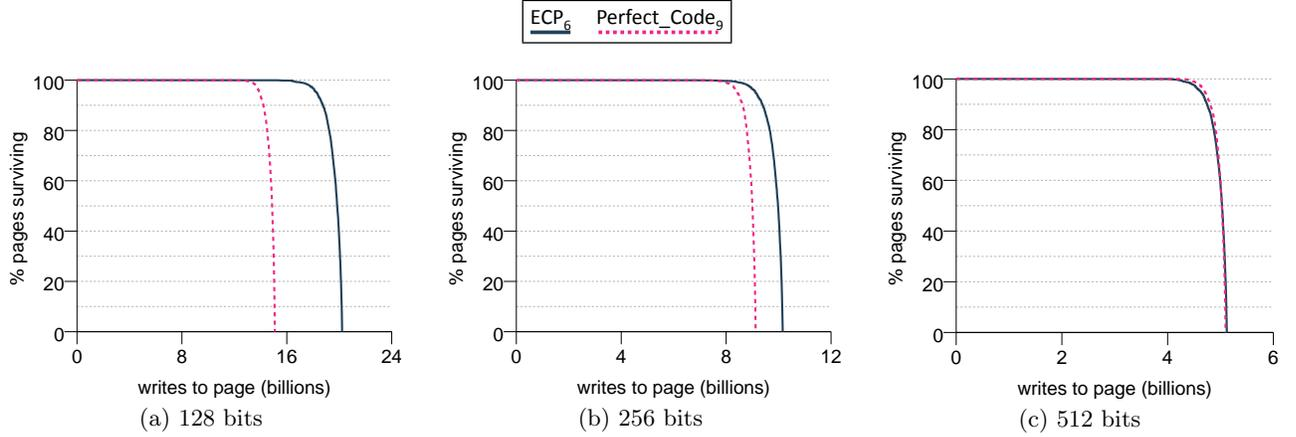
Figure 6: The comparative endurance of Perfect\_Code<sub>9</sub> and ECP<sub>6</sub>, using rotating wear leveling to spread wear evenly over both data bits and correction structures. The graphs assume writes that span (a) 128, (b) 256, (c) 512 bits.
