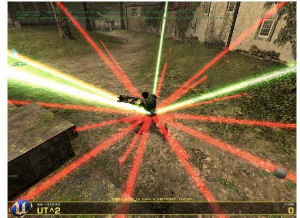
Ray traces for walls/level geometry
