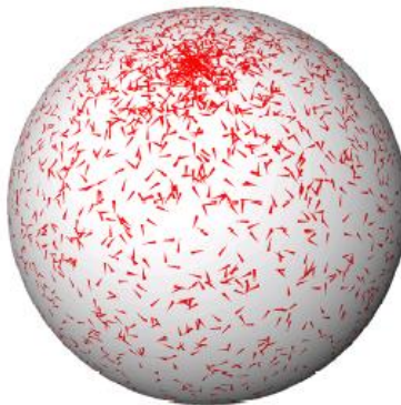
Figure 6.7: A finite set of vectors, generated by uniform sampling in the natural parametrization, depicted as they are distributed on the surface of a sphere. Notice that despite the significant number of points sampled, there are still fairly large pockets uncovered, and correspondingly there are several places where samples are wasted by repetition.
