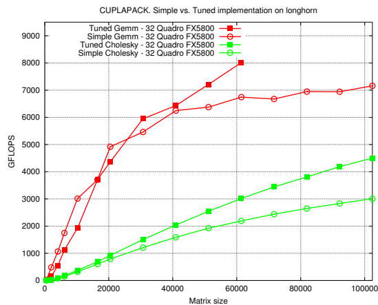
Figure 5: Comparison between the simple and tuned implementation of PLAPACK for the matrix-matrix multiplication and the Cholesky factorization on 16 nodes of LONGHORN (using 32 GPUs).
