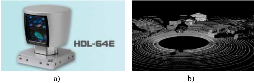
Figure 2.4: a) The Velodyne HDL-64E. b) An example of the data reported by the sensor.
