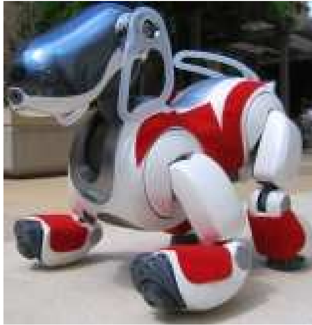
Figure 2.1: The Sony Aibo ERS-7 has four legs that each have three degrees of freedom, three additional degrees of freedom in its neck, and a color camera in its nose.
