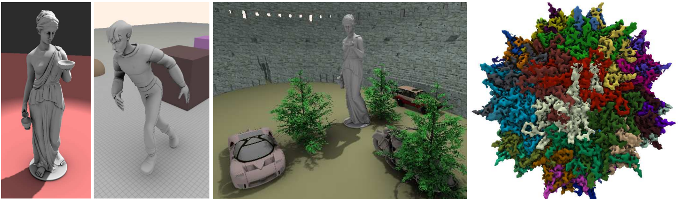
Figure 1: These images illustrate our ambient occlusion approximation running on a modern GPU. Our method can be used for a number of applications including (a) Rendering high-detail models; this model has around 65K triangles. (b) Dynamic/deforming models (that undergo non-rigid deformations) (c) Enhancing natural objects such as trees, and in games where models such as cars are used. This scene currently renders at around 4 fps and has over a million triangles. (d) Realistic rendering of molecular data that provides similar/superior quality to specialized software such as [Bajaj et al. 2004; Tarini et al. 2006].
