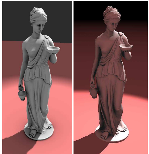
Figure 3: Ambient occlusion generated real-time using our image-space approach (left) at about 7 fps compared with an offline version on the right ([Arikan et al. 2005]) computed in 5 minutes.
