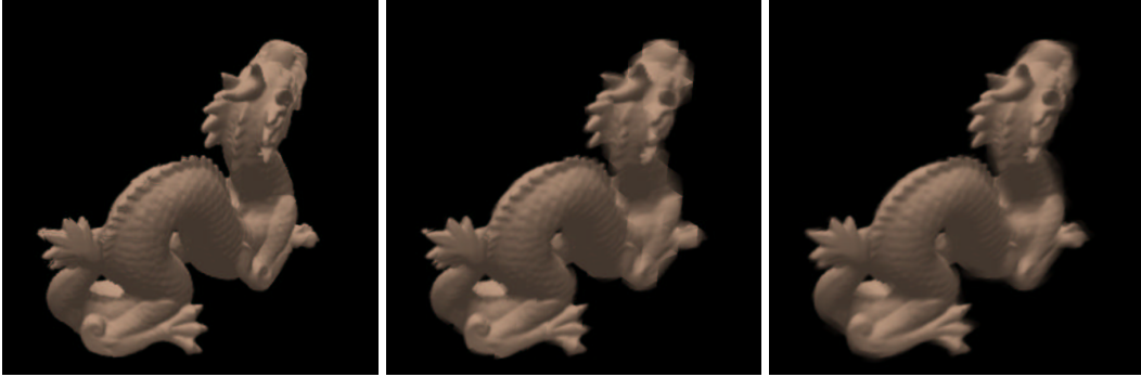
Figure 4.9: A model rendered with different reconstruction kernels. Left , a piecewise constant kernel produces artifacts in the tail, back and front feet of the dragon. Middle , a piecewise linear kernel with small support solves the artifacts in the back, but not in the tail of the dragon. It also introduces very noticeable artifacts in the head and near the front feet of the dragon. This image looks worse than the image on the left. Right , a piecewise linear kernel with large support blurs the artifacts in the tail, front legs and head of the dragon, but it provides a uniform quality representation comparable to the constant kernel.
