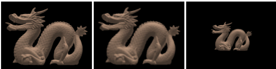
Figure 4.15: The dragon model is used in these images to show how DPP light-field models allow separate control of their positional and directional resolutions. Left , model #1 with 20480 directional samples and 256x256 spatial samples. Middle , model #2 with 81920 directional samples and 128x128 spatial samples. The dragon looks blurrier due to lower spatial resolution. Right , the 81920x128x128 model looking from a distance. The spatial quality is comparable to the first model. Note that both models have the same total number of samples. Geometric model courtesy of Brian Curless and the Stanford Computer Graphics Lab.
