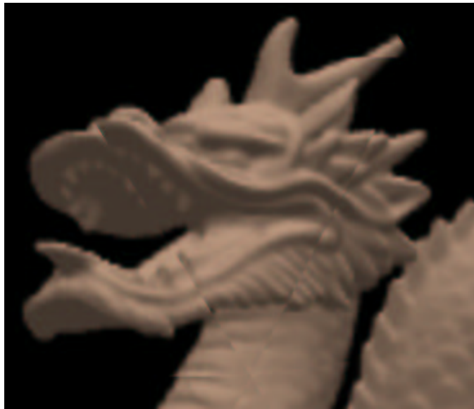
Figure 5.3: Seams in a DPP light-field representation. This image suffers from pixelation artifacts along the bottom lip of the dragon.
