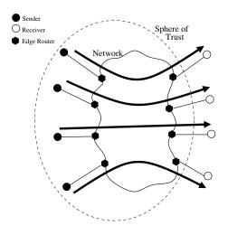
Figure 1: Unicast with untrusted receivers.
