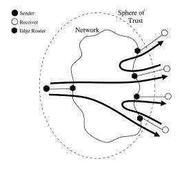
Figure 3: Peer-to-peer multicast with untrusted hosts.
