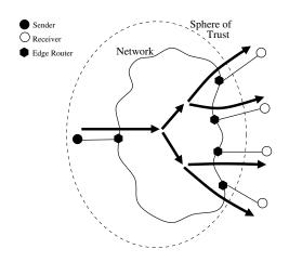
Figure 2: IP multicast with untrusted receivers.
