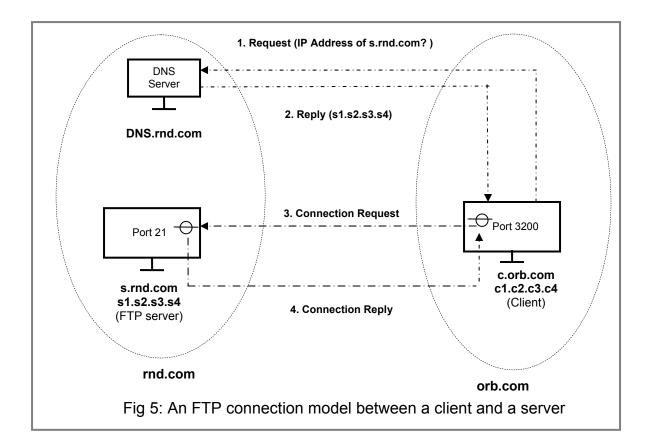
In order for the client and the FTP server to exchange request and reply messages, the client needs to establish a TCP connection to the FTP server. For this purpose, the client should first (a) obtain the IP address of the FTP server, and then (b) send a TCP connection request message to the FTP server. We now discuss these two steps in detail.
