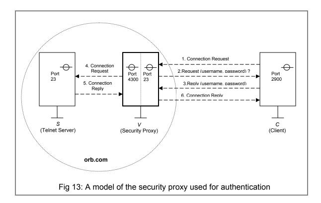
4. On successful authentication of the client, the security proxy chooses a TCP port at random (port number 4300 in this example) and forwards the connection request to the Telnet server. The parameters of the connection request message are as follows:
