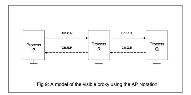
We denote the channel from the process **P** to the process **R** as **Ch.P.R**, while the channel from the process **R** to the process **P** as **Ch.R.P**. Similarly, the channel from the process **R**
