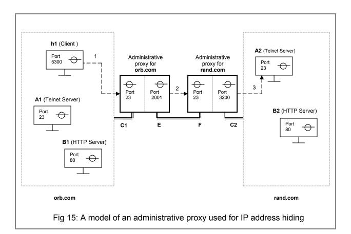
While forwarding the request R, the administrative proxy of the computer network **orb.com** saves certain details about the current connection. This enables it to forward all subsequent replies from the administrative proxy of the computer network **rand.com** back to the client. We represent the information, which is saved by the administrative proxy, as follows.
