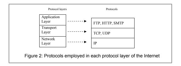
Our classification methodology is analogous to the structure of the Internet protocol hierarchy shown in the above figure. We next discuss the classification and the applications of firewalls followed by a model of the static packet filter firewall.
