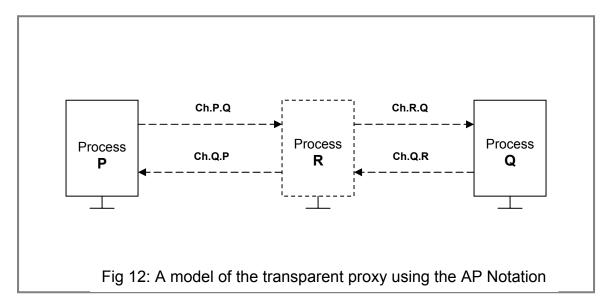
We denote the channel from the process P to the process Q as Ch.P.Q, while the channel from the process Q to the process P as Ch.Q.P. In the above figure, the process R intercepts every message traversing on the channels Ch.P.Q and Ch.Q.P.
