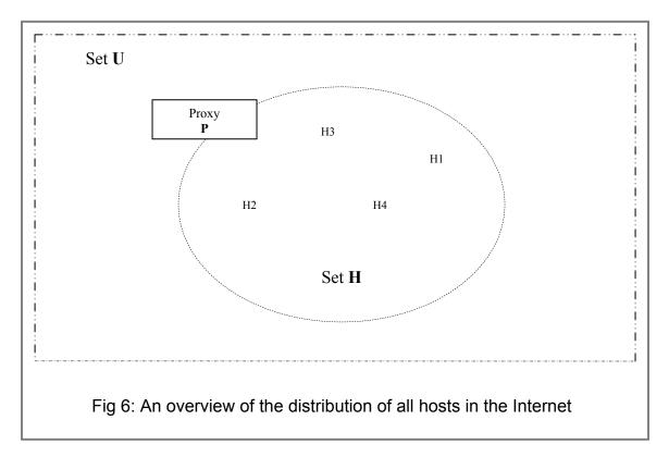
The proxy  $\mathbf{P}$  examines every data packet that goes in or comes out the set  $\mathbf{H}$ . Therefore, the proxy will examine a data packet in the following two cases:
